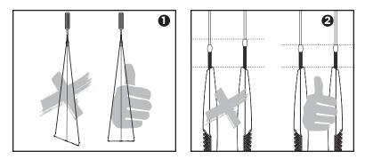
If the bar is not perpendicular to the locking tube, one of the back lines has stretched more than the other. There are two ways to fix this:
