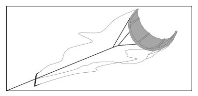
It is important that you inspect you front leader line often for any damage or wear. This is easily done by grabbing the leash attachment ring and pulling the line out from the trim loop system. (This can not be done while lines are wrapped around the bar.)
