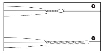
**Warning:** Over tightening the back line trim winding mechanism can result in damage to your bar floats, spring tensioning system, and the winder itself.
